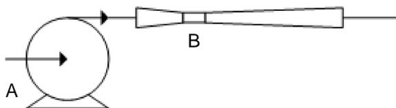
Figure 2. Schematic plan representation: A - pump, B - Venturi ejector
