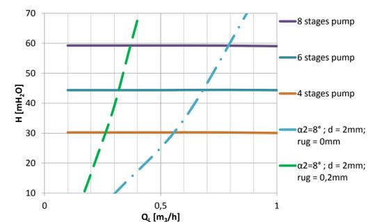
Figure 5. Characteristic curve with (---) / without (- - -) equivalent sand roughness
