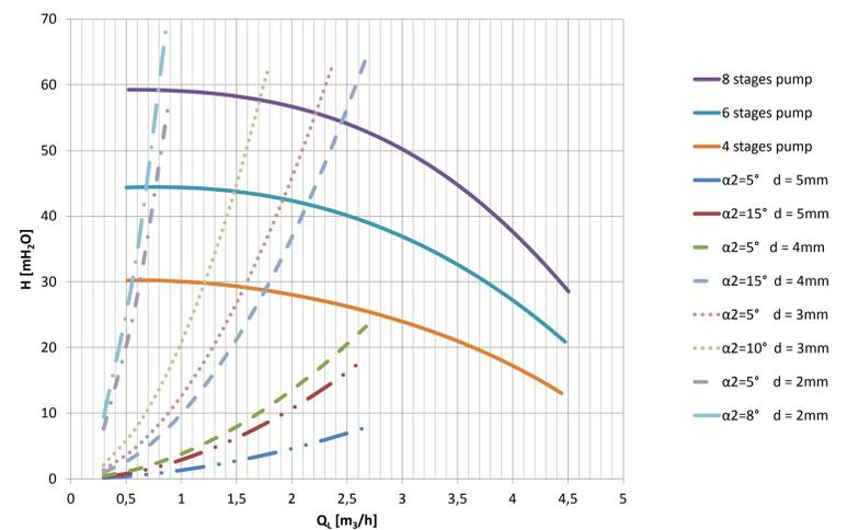
Figure 3. Pump and ejector characteristic curves
