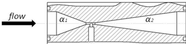
Figure 1. Venturi ejector scheme
