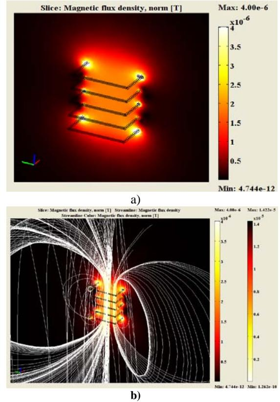
**Figure 9.** a) Slice: Distribution of magnetic flux density, b) Streamline: Distribution of magnetic flux density
