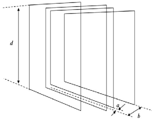
**Figure 3.** Merritt coil system - four square coils.
