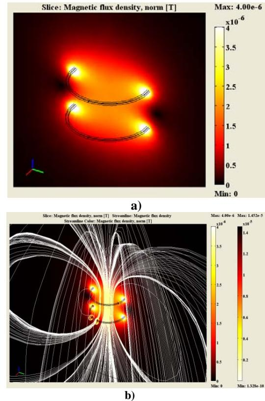
Figure 5. a) Slice: Distribution of magnetic flux density, b) Streamline: Distribution of magnetic flux density.
