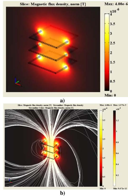
**Figure 7.** a) Slice: Distribution of magnetic flux density, b) Streamline: Distribution of magnetic flux density.
