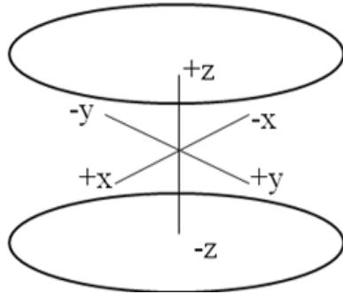
**Figure 6.** Lines to measure and to calculate an equivalent cube of uniform magnetic field in coil system.
