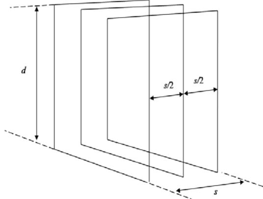
**Figure 2.** Merritt coil system -three square coils.
