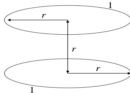
**Figure 1.** Helmholtz system coil.
